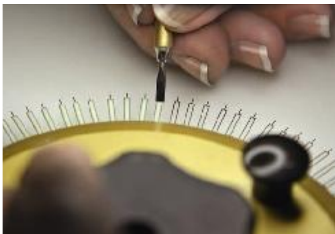
Manually painting Super-LumiNova on the backside of Bathyscaphe hands.
