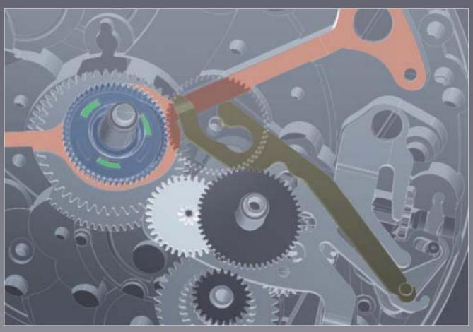
The crown in the time-setting position: clutch disengaged.
