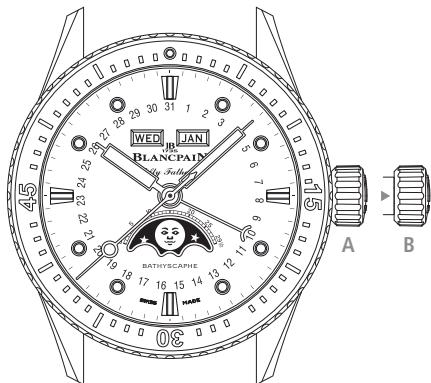
Kindly unscrew the crown (**position A**) before performing any corrections, and screw it in again once the watch has been adjusted.
