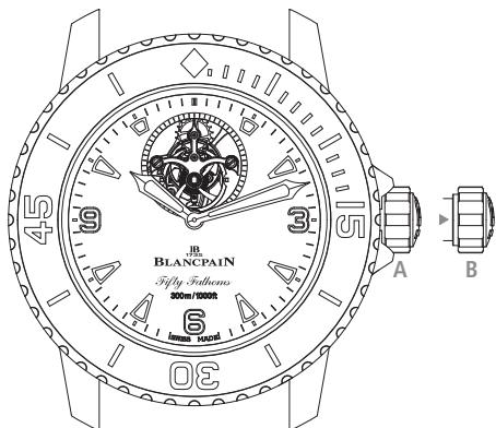
Kindly unscrew the crown (**position A**) before performing any corrections, and screw it in again once the watch has been adjusted.
